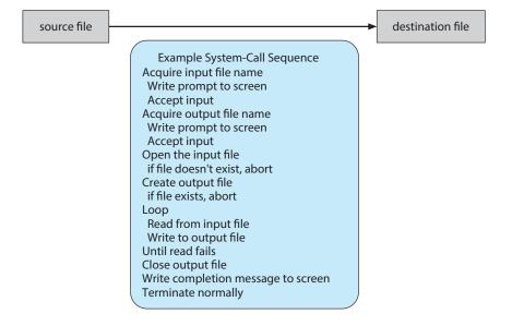
Figure 2.5 Example of how system calls are used.
