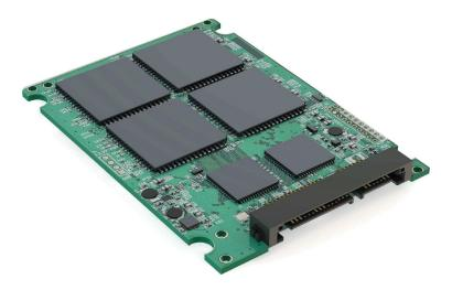
Figure 11.3 A 3.5-inch SSD circuit board.
