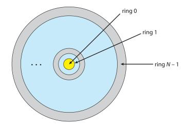
Figure 17.1 Protection-ring structure.
