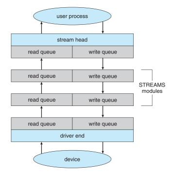
Figure 12.15 The STREAMS structure.
