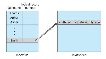
Figure 13.6 Example of index and relative files.
