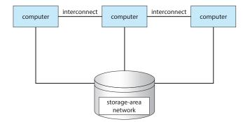
Figure 1.11 General structure of a clustered system.
