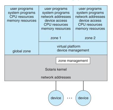
Figure 18.7 Solaris 10 with two zones.
