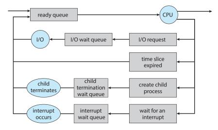
Figure 3.5 Queueing-diagram representation of process scheduling.
