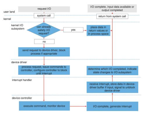
Figure 12.14 The life cycle of an I/O request.
