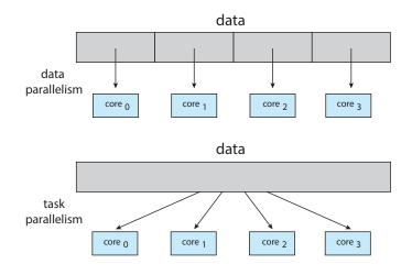
Figure 4.5 Data and task parallelism.
