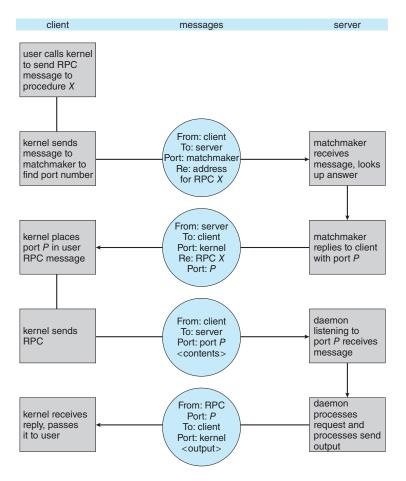
Figure 3.29 Execution of a remote procedure call (RPC).
