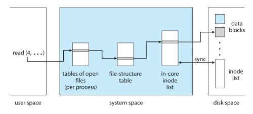
Figure C.8 File-system control blocks.
