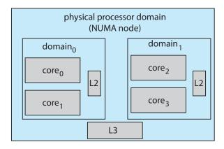
Figure 5.27 NUMA-aware load balancing with Linux CFS scheduler.
