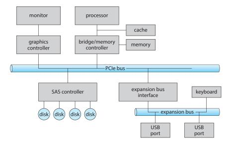
Figure 12.1 A typical PC bus structure.
