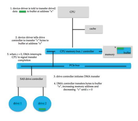
Figure 12.6 Steps in a DMA transfer.
