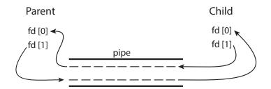
Figure 3.20 File descriptors for an ordinary pipe.
