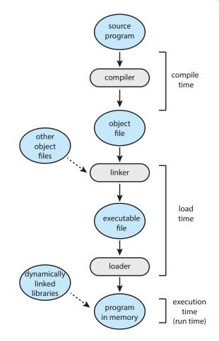
Figure 9.3 Multistep processing of a user program.
