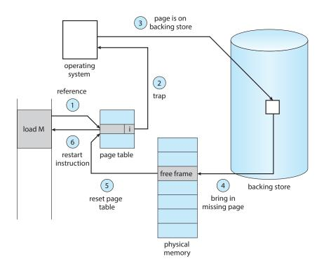
Figure 10.5 Steps in handling a page fault.
