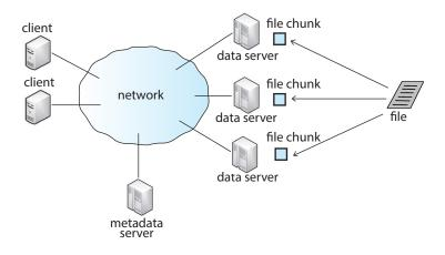
Figure 19.13 An example of a cluster-based DFS model
