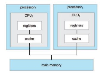
Figure 1.8 Symmetric multiprocessing architecture.
