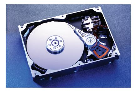
Figure 11.2 A 3.5-inch HDD with cover removed.
