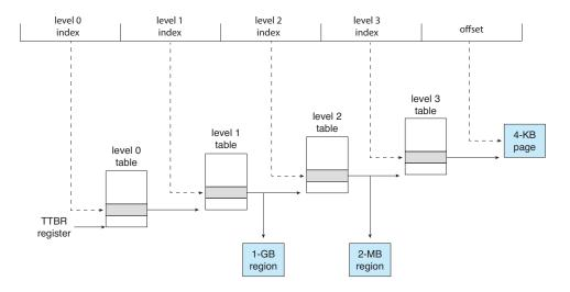
Figure 9.27 ARM four-level hierarchical paging.
