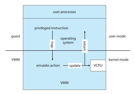
Figure 18.2 Trap-and-emulate virtualization implementation.
