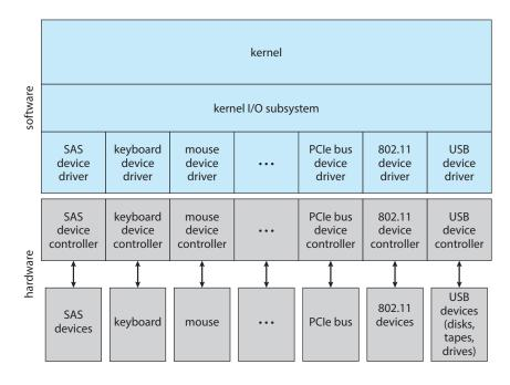
Figure 12.7 A kernel I/O structure.
