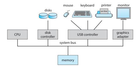
Figure 1.2 A typical PC computer system.
