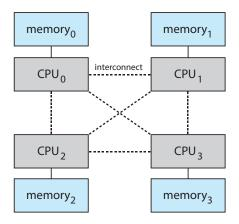
Figure 1.10 NUMA multiprocessing architecture.
