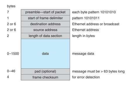
Figure 19.9 An Ethernet packet.
