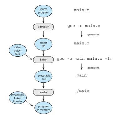
Figure 2.11 The role of the linker and loader.
