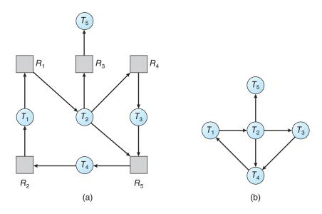
Figure 8.11 (a) Resource-allocation graph. (b) Corresponding wait-for graph.
