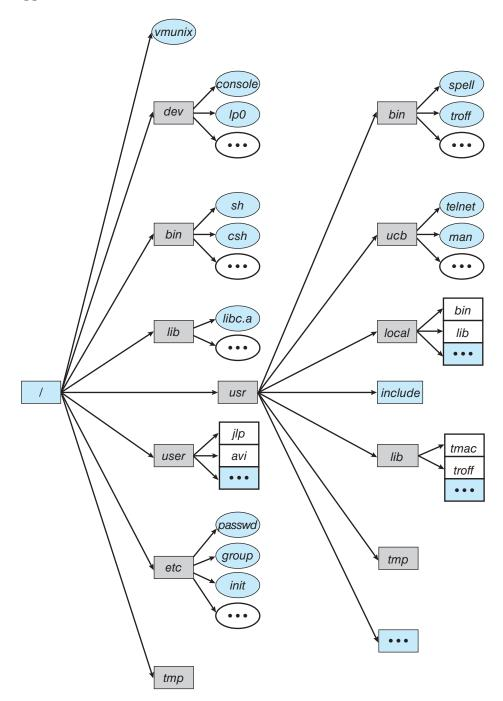
Figure C.3 Typical UNIX directory structure.
