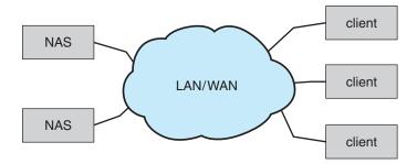
Figure 11.12 Network-attached storage.
