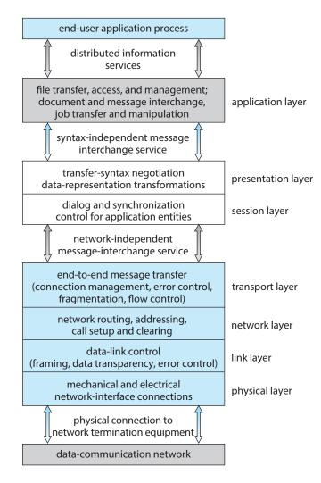
Figure 19.6 The OSI protocol stack.
