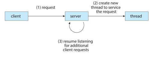
Figure 4.2 Multithreaded server architecture.
