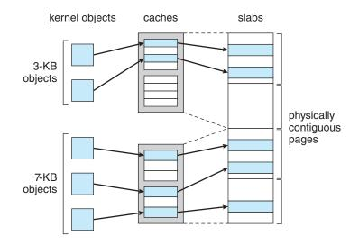
Figure 10.27 Slab allocation.
