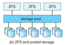
Figure 11.18 Traditional volumes and file systems compared with the ZFS model.
