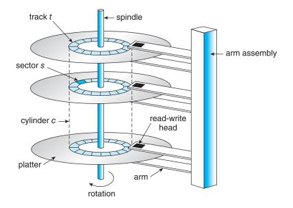
Figure 11.1 HDD moving-head disk mechanism.
